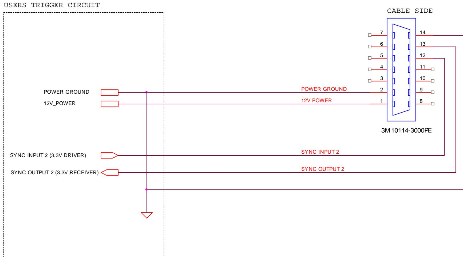
The non-isolated trigger circuit is connected to a Texas Instruments SN74LVC2G241 buffer/driver inside the camera. The required sync input current is less than 10uA and the maximum sync output current is 24mA. See the Texas Instruments SN74LVC2G241 for more detailed information.
