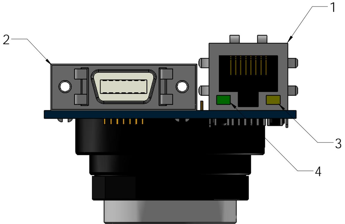
Figure 1. GB SERIES connection diagram.
