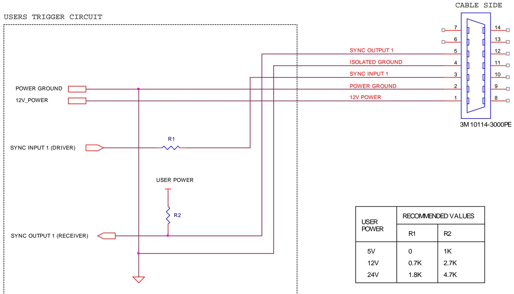
This circuit assumes a 10mA drive current ( $I_F$ ) from User's trigger circuit into camera through R1. R2 is connected to the open collector of Fairchild MOCD207. The corresponding transistor emitter is connected to isolated ground. See the Fairchild MOCD207 datasheet for more detailed information.
