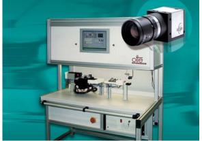
Up to 15 high-resolution color cameras check the installed plugs, fuses and relays on the wiring harnesses
